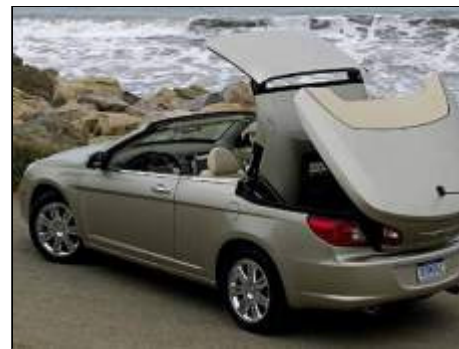
THIS IS HOW IT WORKS: The Chrysler Sebring convertible's three-piece steel roof is stacked the boot when down rather than the Z-fold of BMW 3-Series convertible.
